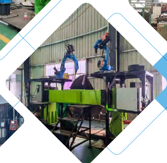
04 斗顶自动化焊接 Automatic welding of bucket top
